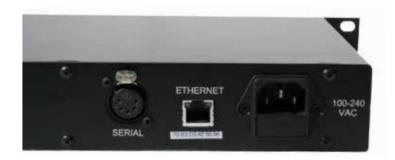
The self-contained master controller system incorporates a power supply, manual switches and CPU running software in a 1 space rack mount package. It allows communication with Servoreelers and external controllers (Crestron, AMX, etc.). The unit has an Ethernet connection (IEEE 802.3), serial connection (RS-232), and an array of non-Ethernet RJ45s (one or two groups of six, 6 or 12 total) which transmit 24 volt power and control signals to individual Servoreelers.
